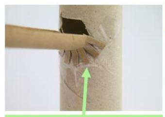
The ends of the cardboard tube are shaped and small cuts are made to help the tube to fan out and accurately fit the other tube.
